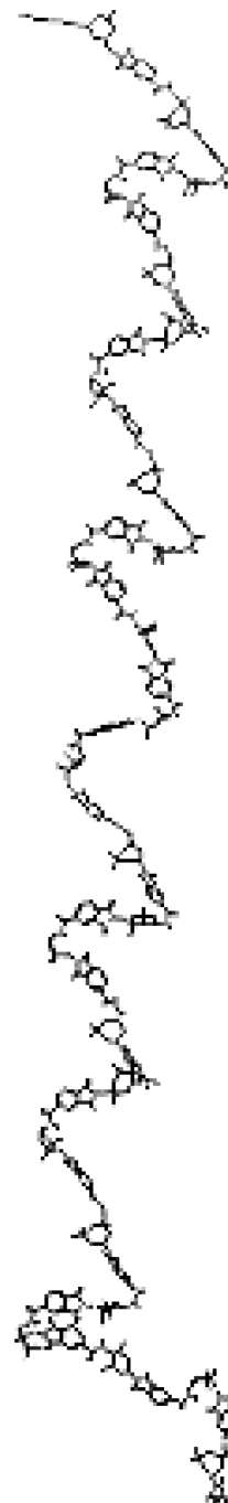
Fig. 1. Energy minimized chain structure of poly(amide-imide) (PAI-1) based on isophorone diisocyanate (IPDI) and trimellitic anhydride (TMA).
